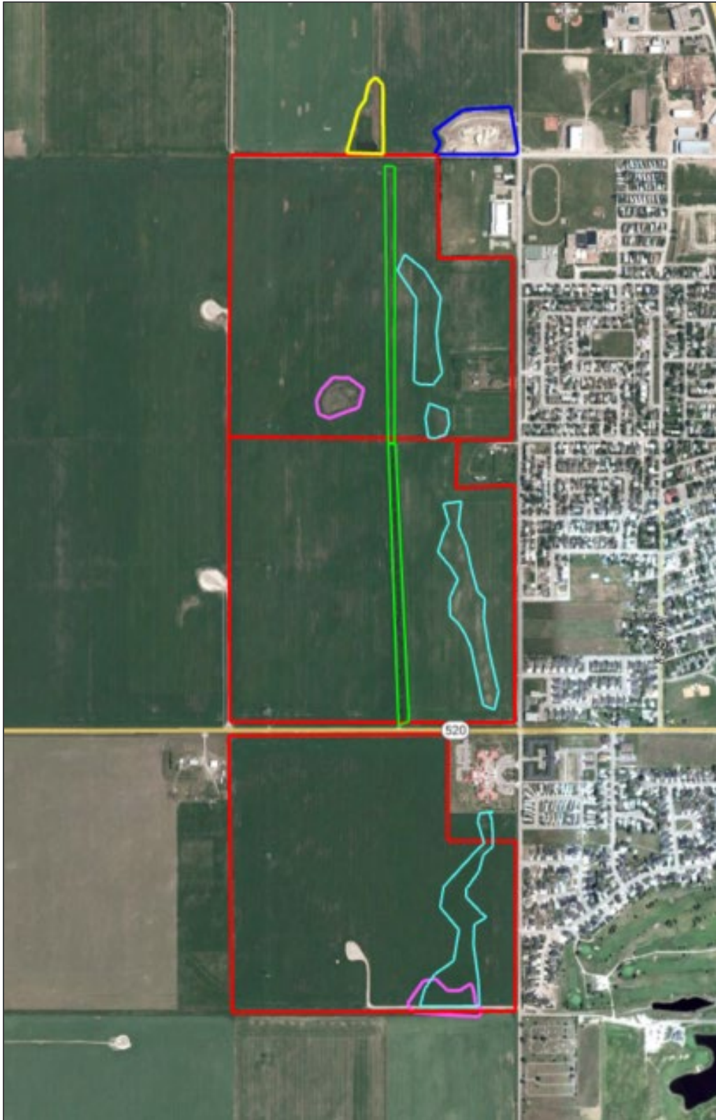
Figure 4: Potential wetland boundary (pink), dugouts (yellow), ephemeral draws/wet areas (light blue), stockpile area (dark blue), shelterbelt (green) and project boundary (red) (Google Earth Pro, 2025).
